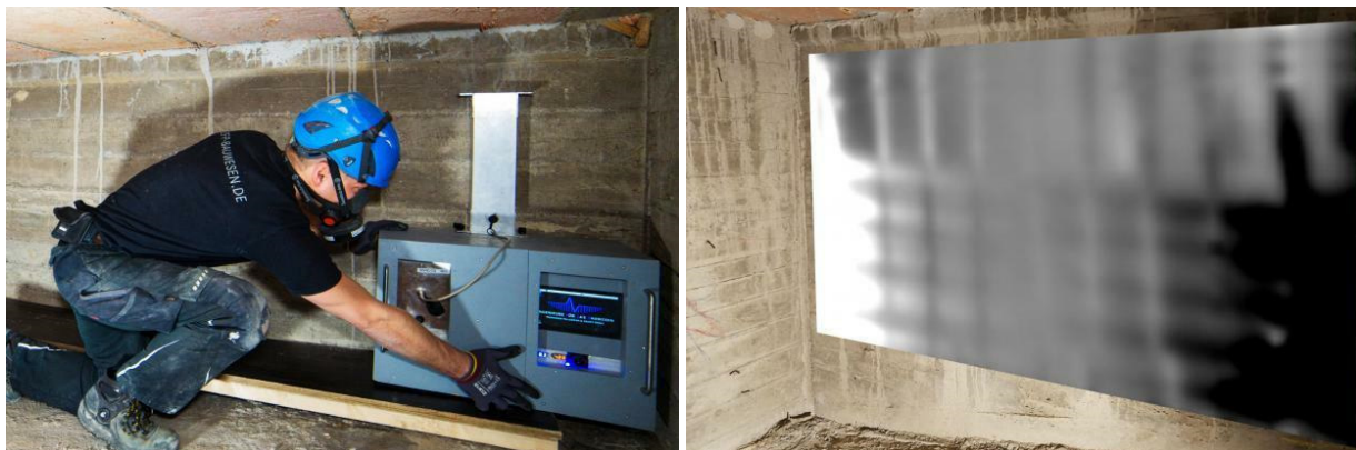
Figure 3: Measurement with the GreyOne - Sensor Unit (left), magnetic image of longitudinal tendons (right)
