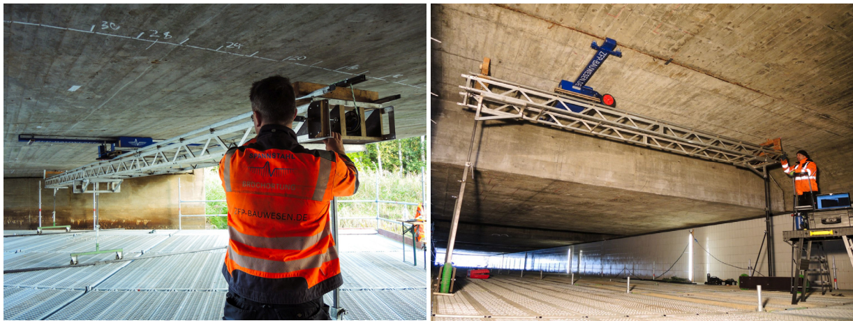
Figure 5: Investigation of prestressed bridge surfaces with the BlueOne – Sensor Unit
