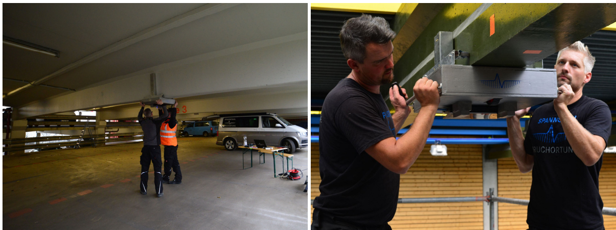
Figure 4: Investigation of prestressed concrete beams with the U - Sensor Unit
